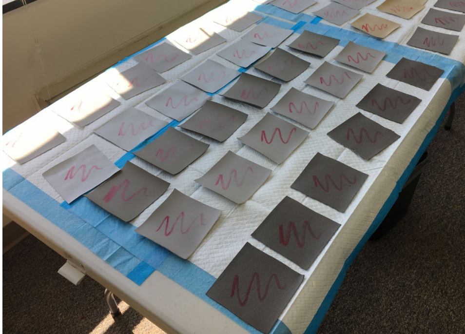
APPLICATION OF STAIN, 48 HR DWELL TIME
